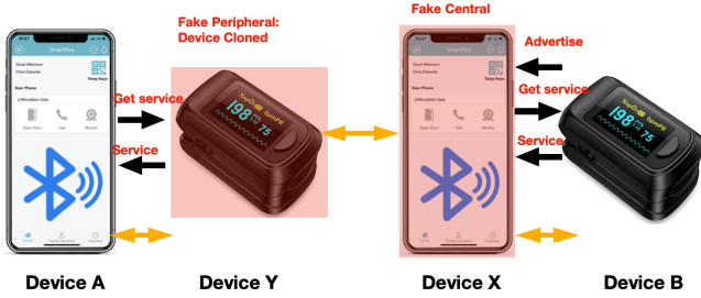
Figure 1: BLE Man-in-the-Middle (MITM) Attack
